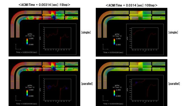
I calculated the original Case files which the uniformFixedValue type is not applied to any boundary conditions and the special decomposition options is not used. Then, the pressure discontinuities have disappeared.
